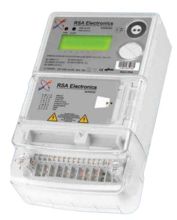
• A Digital Energy (Electricity) Meter which is an active and reactive multi tariff device that measures and stores consumed energy and other parameters required by the energy utility companies.
